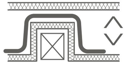
LAME D'AIR INTERMÉDIAIRE AUTOMATIQUEMENT RÉALISÉE
